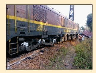
The position of the locomotive is such that its one wheel was locked in the track and once it was tried a little bit left from rear, the other side was in tilted condition started further down, so it was clear that loco cannot be worked out with one crane so it was also waiting for KRDL crane to come and assist.
