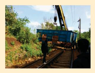
For tackling the 50<sup>th</sup> wagon again track linking was required, which started at 3:20 hrs and given at 7:00 hrs. 120T crane was brought inside the tunnel at 7:10 hrs. The trolley of 49<sup>th</sup> wagon grounded at 7:40 hrs and 8:10 hrs. The 50<sup>th</sup> wagon was then hold on the crane hook from one end and pulled out of the tunnel and grounded at 10:15 hrs. The two trolleys of the wagon were grounded at 10:45 hrs and 11:00 hrs respectively.
